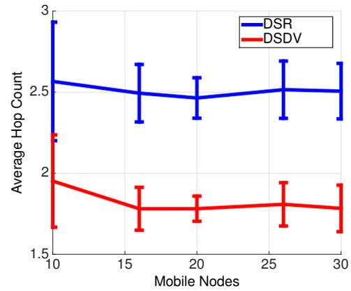
Fig. 10. Average hop count as a function of mobile nodes number.
