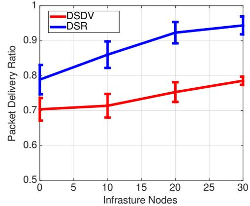
Fig. 4. Packet delivery ratio with low mobility (600 seconds pause time) environment as a function of infrastructure nodes number.
