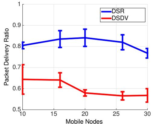
Fig. 7. Packet delivery ratio as a function of mobile nodes number.
