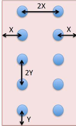
Fig. 11. An example for a deployment of 30 infrastructure nodes of a  $6 \times 5$ .
