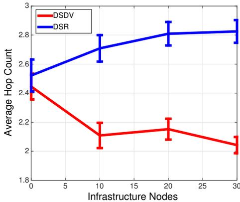
Fig. 6. Average hop count with low mobility (600 seconds pause time) environment as a function of infrastructure nodes number.
