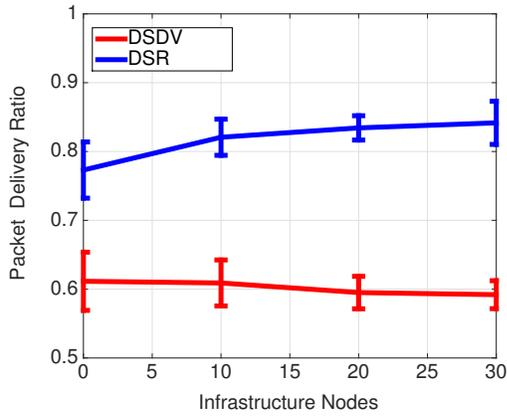
Fig. 3. Packet delivery ratio in high mobility (0 seconds pause time) environment as a function of infrastructure nodes number.
