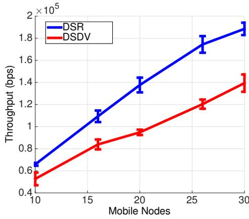
Fig. 8. Throughput as a function of mobile nodes number.
