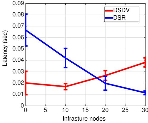
Fig. 5. Mean Latency in low mobility (600 seconds pause time) environment as a function of infrastructure nodes number.
