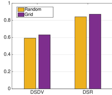
Fig. 13. Packet delivery ratio with 30 infrastructure nodes placed randomly or in grid.
