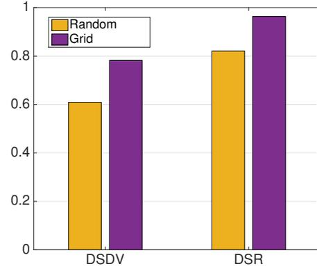
Fig. 12. Packet delivery ratio with 10 infrastructure nodes placed randomly or in grid.
